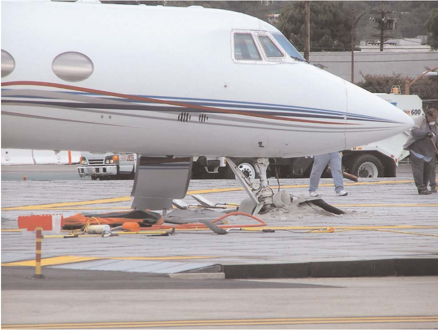
EMAS is a good alternative if a 240m RESA is not available. At geographically and topographically challenged airports where the system has been installed a number 'saves' have taken place of aircraft from a GIII and SF340 up to a 747-200F.
