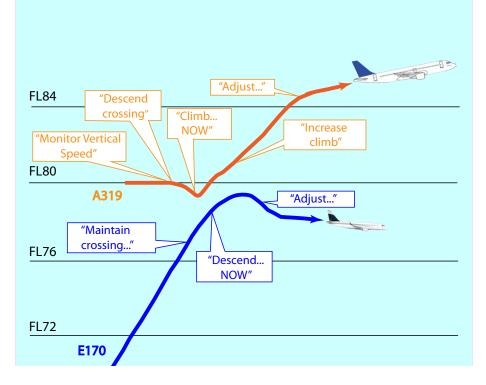
provide sufficient vertical spacing and generates reversal RAs: a reversal descent ("Descend, descend NOW") RA for the climbing E170 and a reversal climb ("Climb, climb NOW") RA for the descending A319. Both pilots respond to the reversal RAs.
