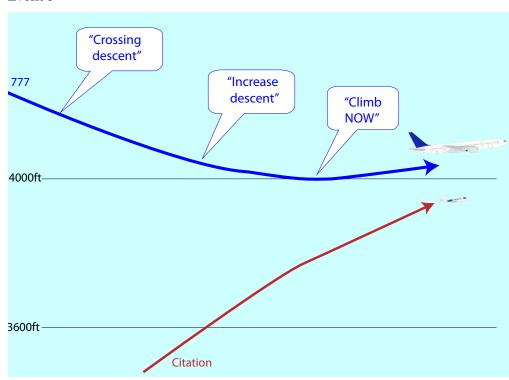
Cessna Citation is on the ground requesting start up departure and clearance. The Citation is not equipped with TCAS II. Its maximum take-off mass is below 5700 kg, so the aircraft is outside the current equipage mandate. The tower controller clears the Citation to climb to 3000 ft after take-off. The pilot reads back "4000 ft" and this incorrect read-back is not detected by the controller. Consequently, once airborne the aircraft is climbing to 4000 ft.
