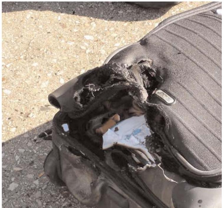
Once ignited, a battery fire may be difficult to extinguish, reigniting several times before being fully controlled.
