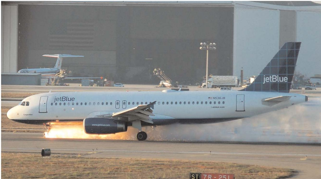
The recent incident in the United States where a Jet Blue A320 landed in Los Angeles with the nose wheels turned 90 degrees has caused increasing concern among pilots and operators of Airbus A320 family aircraft. Through contacts at Airbus, IFALPA has learned that over the past 10 years, there have been 13 similar events worldwide, with four different causes identified. The summary below is a discussion of the cause factors for each event, and the solutions that Airbus has implemented:
