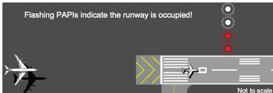
Figure 1. Final Approach Runway Occupancy Signal (eFAROS)
