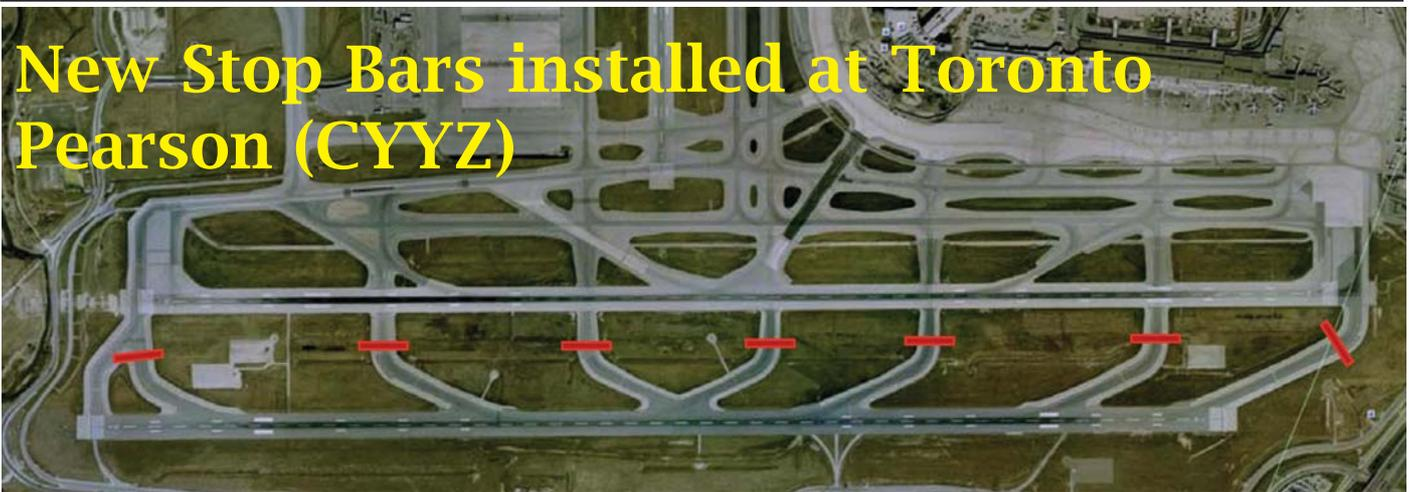
The stop bars will be installed on the rapid exit taxiways leading from runway 06R/24L as they approach runway 06L/24R. Nav Canada advise that the stop bars, which will be operated by tower controllers, may not always be in use when the airport configuration requires the use of this closely spaced runway pair. Crews must not assume that the absence of illuminated stop bar is clearance to cross 06L/24R.
