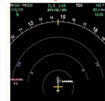
BTW arming by ABRK rotary switch. The Runway LDA must be cross-checked with charts
