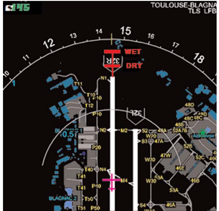
In the event that the aircraft approach path means that the DRY stop line moves beyond the LDA then the track line changes to red and a red "RWY TOO SHORT" visual cue is displayed on the PFD combined with a "RUNWAY TOO SHORT" aural cue
