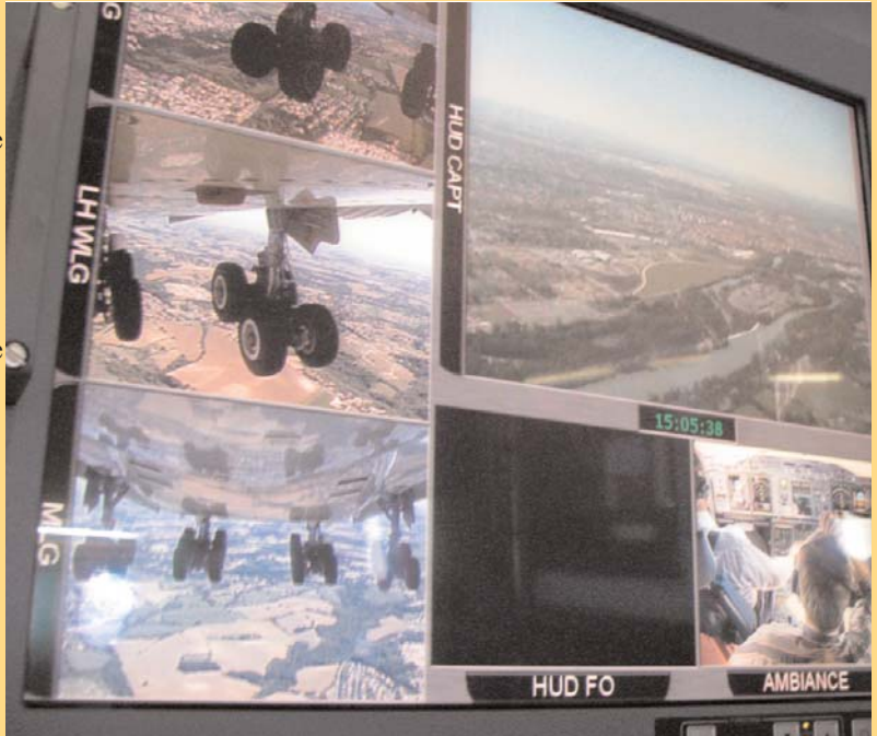
In order to facilitate brake cooling between landings the gear was left down for much of the circuit
