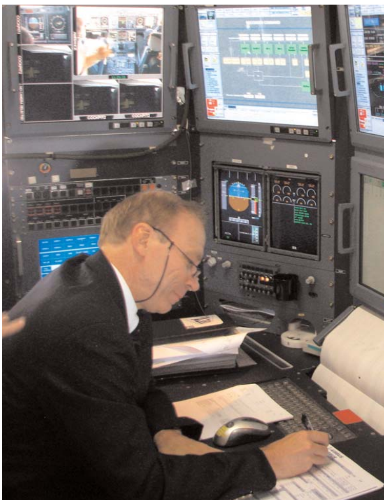
As well as monitoring aircraft systems and performance the Engineering station on F-WWOW can generate phantom TCAS targets for test and evaluation purposes.
