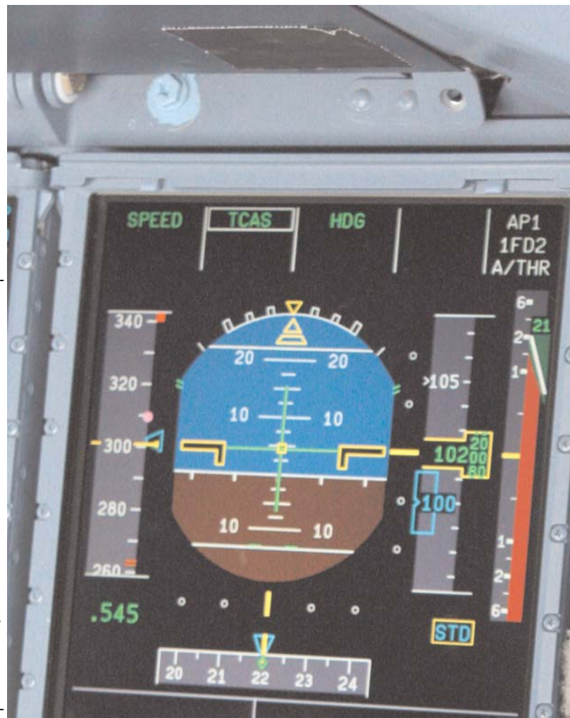
The the VS is bang on the optimal avoidance rate indicated by red/green zones on the VSI and all you have to do is follow the FD.
