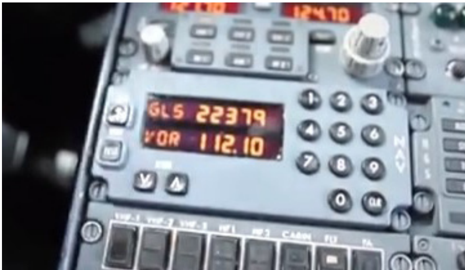
A multi-mode receiver panel on a B737-800
