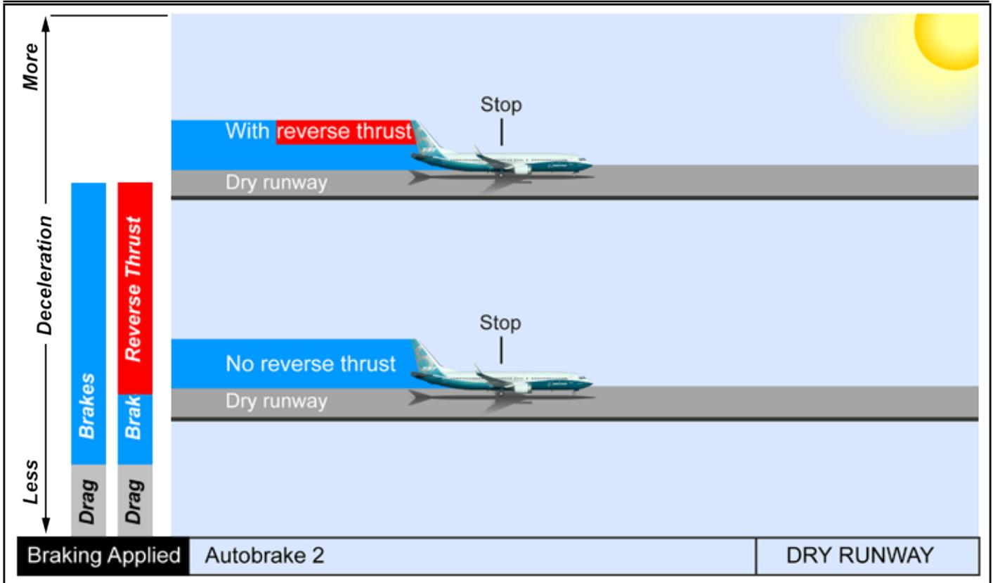
Fig 4: Impact on brake energy using rev thrust with autobrakes
