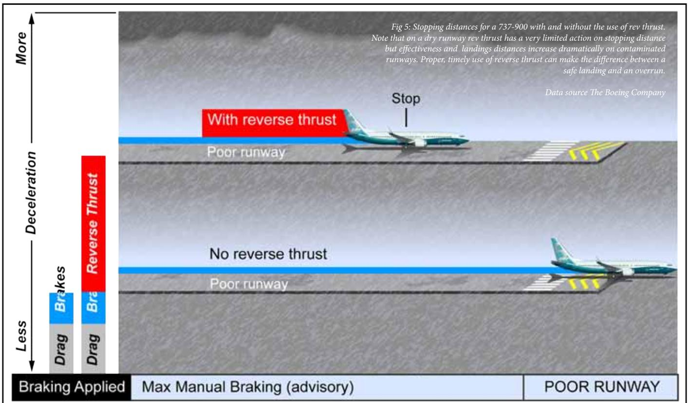
data section in the Quick Reference Handbook (QRH) and consider the landing distance adjustments with and without reverse thrust.
