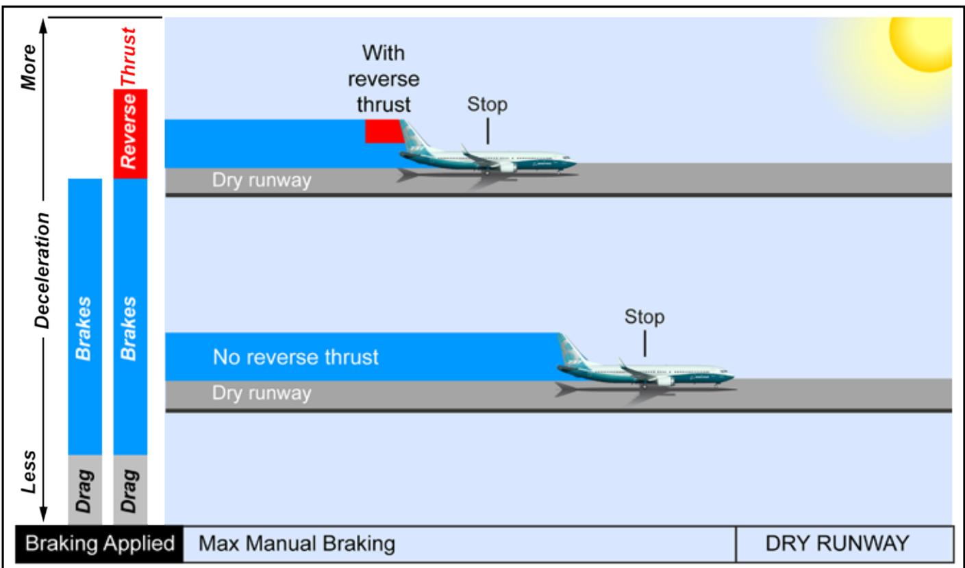
Fig 3: Ratio of stopping forces Data source The Boeing Company
